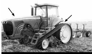
Machine Serial Number Location 8000T Series (Top of final drive case RH side, next to implement valve stack) 8RT Series (Tag is mounted on the RH frame rail)
